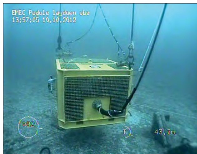
Figure 10.15. The European Marine Energy Centre (EMEC)'s Integrated Monitoring Pod (IMP) during deployment under the Energy Technologies Institute (ETI)'s Reliable Data Acquisition Platform for Tidal (ReDAPT) project. (Photo courtesy of EMEC)
