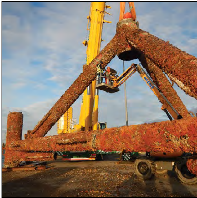
Figure 6.3. Heavily colonized tripod of a decommissioned tidal turbine in the Orkney Islands, Scotland (left), and 25 x 25 cm quadrat showing a close-up of the biofouling organisms, mainly barnacles, sponges, and brittle stars (right). (Photos courtesy of Andrew Want, Heriot-Watt University)
