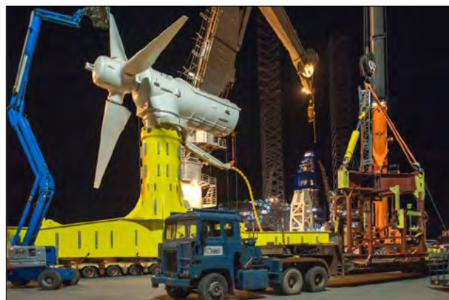
Figure 3.2. A MeyGen tidal turbine ready for deployment in the Inner Sound of Pentland Firth in Scotland. (Photo courtesy of SIMEC Atlantis Energy)
