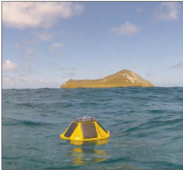
Figure 7.4. Spotter (Sofar Ocean) real-time wave measurement buoy. (Photo courtesy of Grace Chang)
